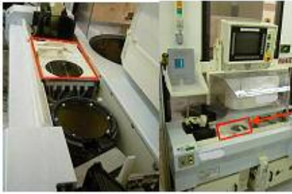
Fig. 2 Wet NovaScan 210 integrated onto a Westtech 372
